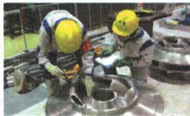
Inspection of a low-pressure condensate pump
